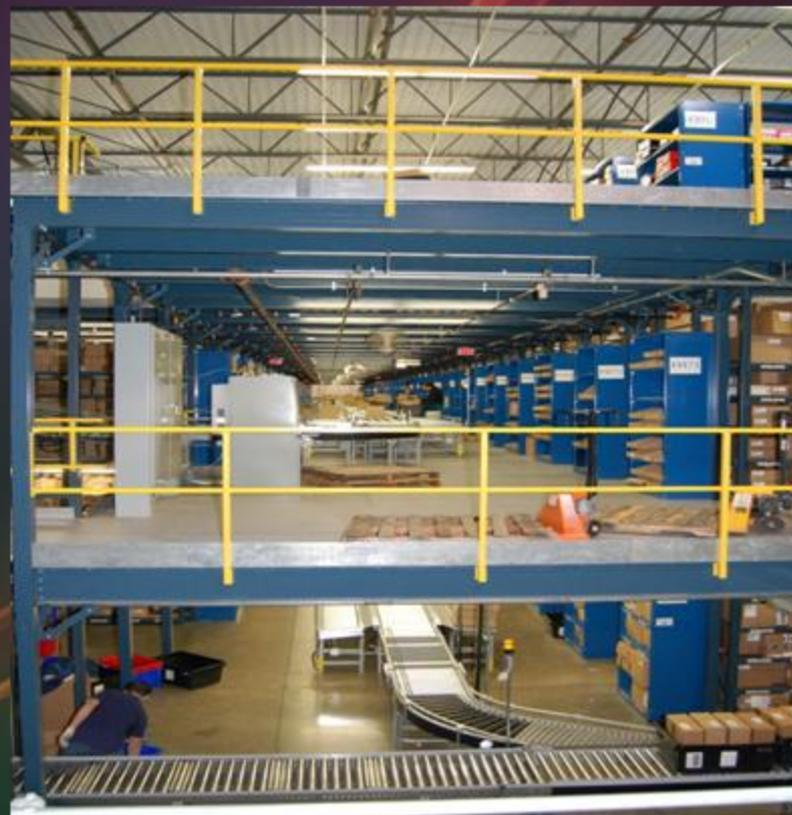
*Recent addition of mezzanine binning maximizes density within an established conveyorized zone pickpath at DART's Midwest fulfillment facility.*
